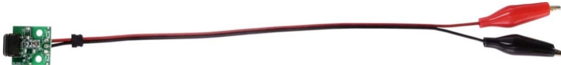
LMPS-mUSB1 - Laser Module Power Supply Board, Input: micro USB, Output: 5 VDC 2A.
